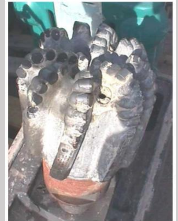
Point Specialized Bit (PDC-PQ 2 ) Bit Used on Point RSS See Drilling Dynamics
